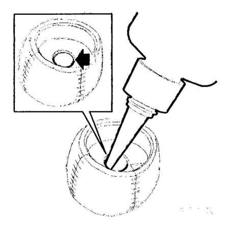
2. Fit the knob to the gear lever. Make sure the spring and foam ring are correctly situated.
