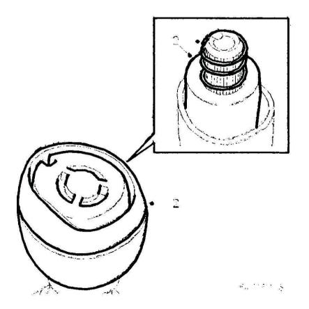
Fit the emblem on the gear lever knob. Do not operate the lever until the adhesive has dried (approx. 30 min).
