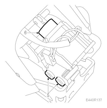
6. Remove the lever from the top of the electromagnet and remove the electromagnet.
