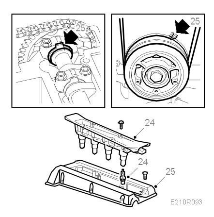
25. Remove the camshaft cover, line up the crankshaft pulley's mark with the timing cover and check that the camshafts are in line with their timing marks.
