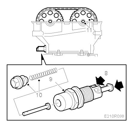
9. Fit the chain tensioner, using a 27 mm socket.
