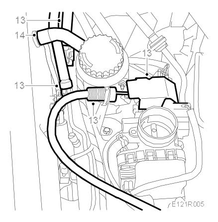
14. Remove the crankcase breather nipple from the timing cover.
