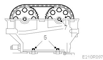
Tightening torque 22 Nm (16 lbf ft).
