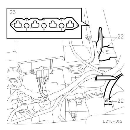
23. Remove the intake manifold with partition. Move the manifold rearwards towards the bulkhead. The lower/centre retaining bolts may be more easily accessible from underneath. Leave the intake manifold in the car.
