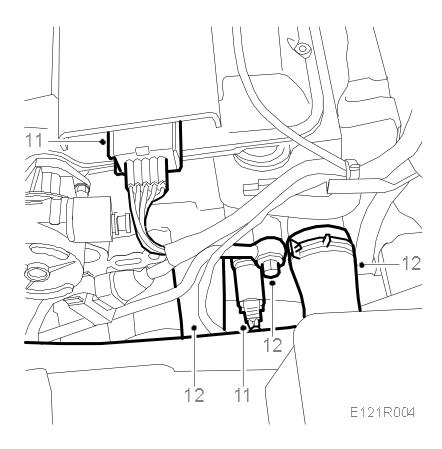
12. Remove the coolant hoses from the cylinder head.
