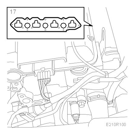
17. Tighten the intake manifold, using a torque wrench.
