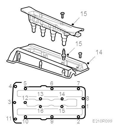
14. Coat the opening in the camshaft cover thinly with oil and fit the cover, starting at the opening. Make sure that the cables at the edge of the cover against the intake manifold do not get trapped. Then tighten the bolt located furthest to the front at the timing chain end. After that, continue all the way round on both the inside and outside.
