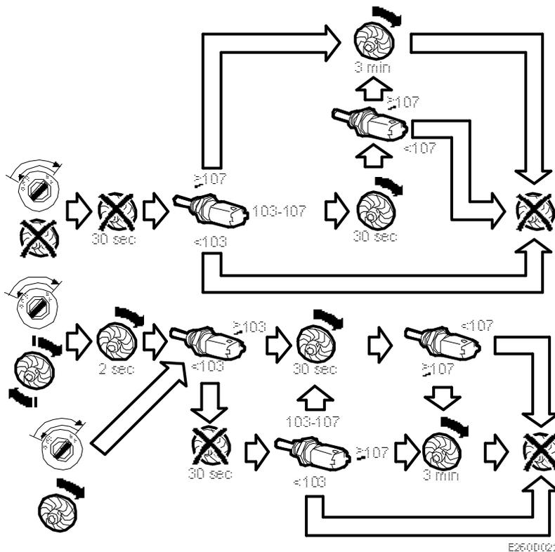
The DICE receives information on the coolant temperature from TRIONIC with the ignition OFF, after 30 seconds and after 1 minute when the ignition switch is in the OFF position.
