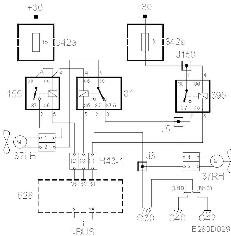
The radiator fans can be run at two speeds, depending on coolant temperature, A/C pressure, car speed and outside temperature:
