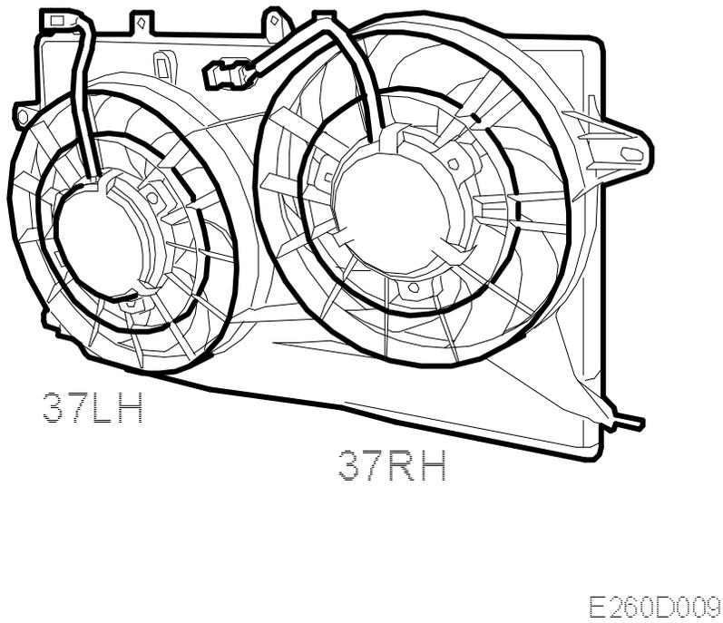
Cars with A/C are fitted with two electric fans mounted behind the radiator. The fans have two
