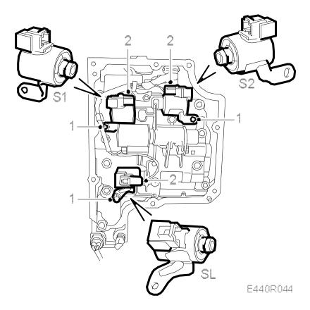
1. Position the solenoid and tighten the bolt.
