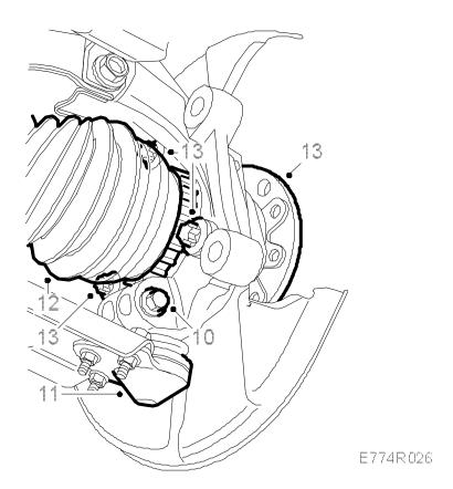
12. Tap out the drive shaft from the hub and lift the hub and steering swivel member from the shaft.
