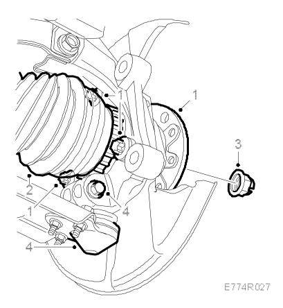
1. Clean the contact surfaces and fit the brake shield and hub with three bolts.
