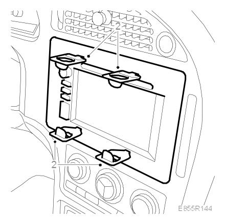
**Cars without navigation**: Remove the plugs carefully to avoid damaging the unit. Remove the screws. Pull out the unit.
