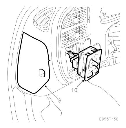
10. Remove the light control panel and unplug the connector.
