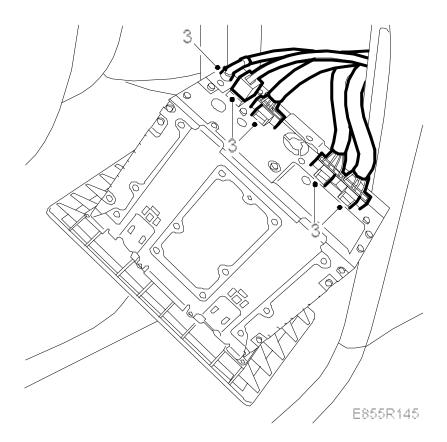
4. **Cars with navigation**: Remove the radio compartment.
