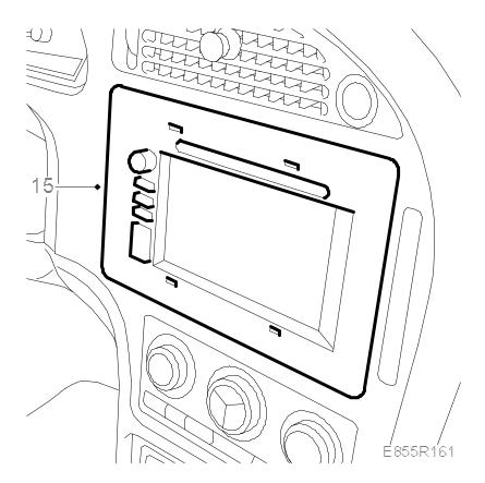
**Cars without navigation**: Fit the screws. Fit the plugs, make sure that the plugs are guided into the grooves.
