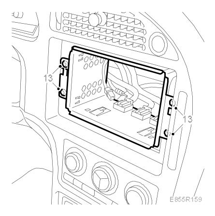
14. Plug in the radio unit's connector.
