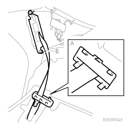
3. Thread the belt through the C-pillar and fit the seatbelt guide (A).
