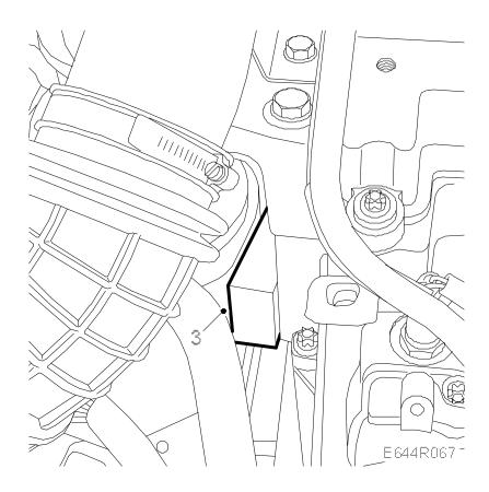
4. Remove and unplug the A/C compressor connector. Use a pair of angled needle nose pliers.
