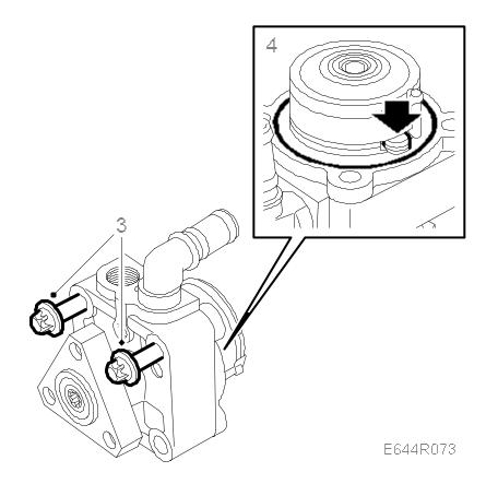
4. Hold in the sprung with one finger and fit the pump to the bracket.
