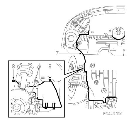
8. Remove the right-hand side cover and wing liner.
