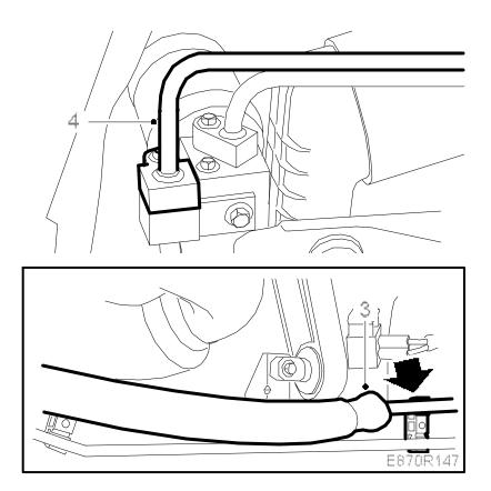
1. Position the high-pressure pipe in the engine bay.
