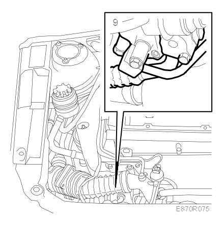
10. Detach the pipe from the receiver and plug the openings.
