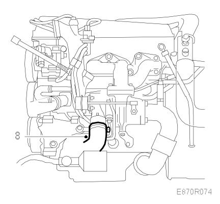
9. Detach the high-pressure hose from the compressor and plug the openings.
