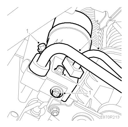
2. Replace the O-rings and lubricate with acid-free vaseline, part no. 30 06 665. Then fit the A/C pipes' PAD connections to the condenser and receiver.
