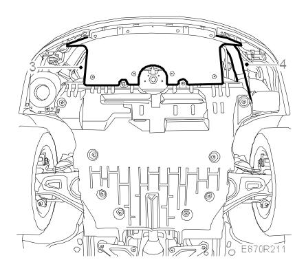
4. **Cars with cooling pipe**: Remove the front cooling pipe from the battery cover.
