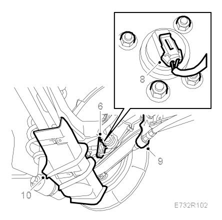
9. Fit the attachment for the parking brake wire.
