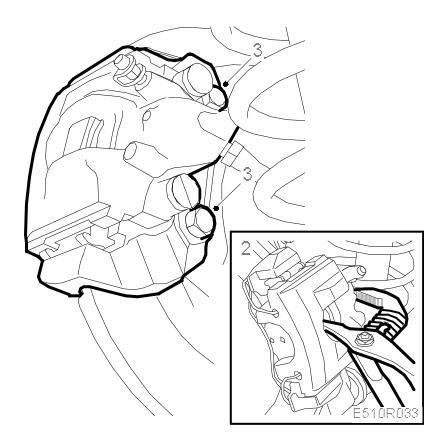
3. Remove the brake caliper and hang it up.
