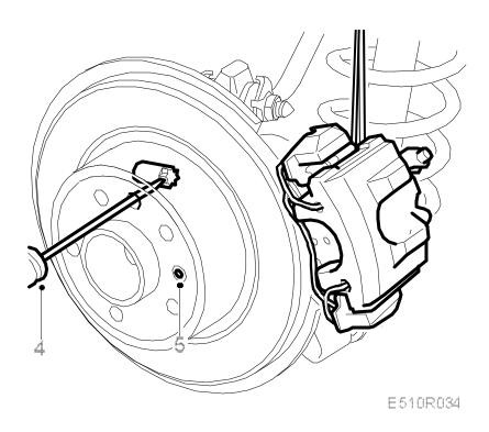
5. Fit the brake caliper. Use Loctite 242, part no. 74 96 268, on the bolts.
