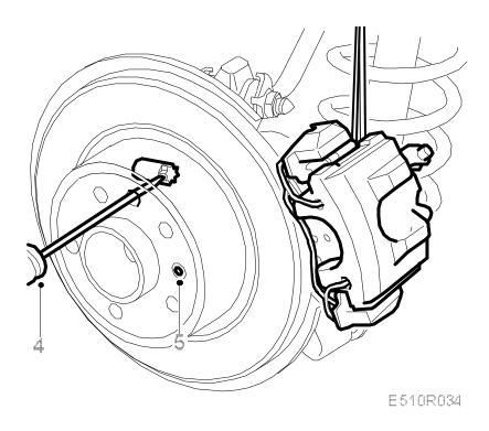
5. Remove the brake disc retaining bolt. Remove the brake disc.
