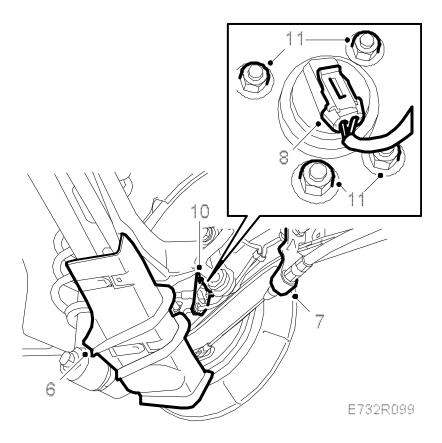
7. Fit the wheel sensor cable in the attachment.
