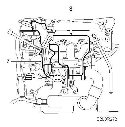
8. Fit the exhaust manifold heat shield.
