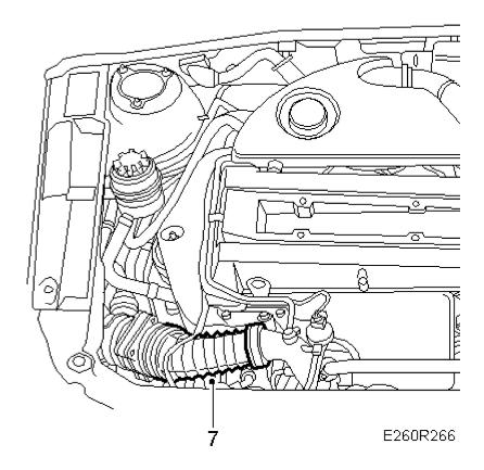
8. Detach the crankcase ventilation pipe from the turbocharger intake manifold and the camshaft cover.
