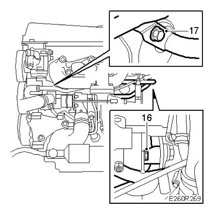
17. Detach both coolant pipes from the coolant pump.
